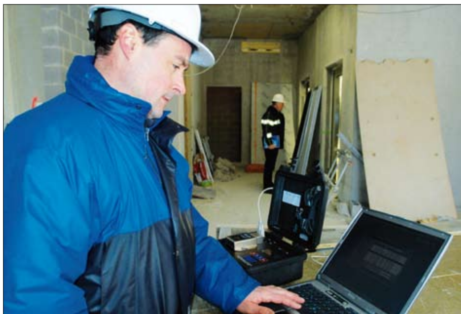
The testing of a lift with actual iron loads, to check traction or brake efficiency can effectively be replaced in many instances by computer testing
